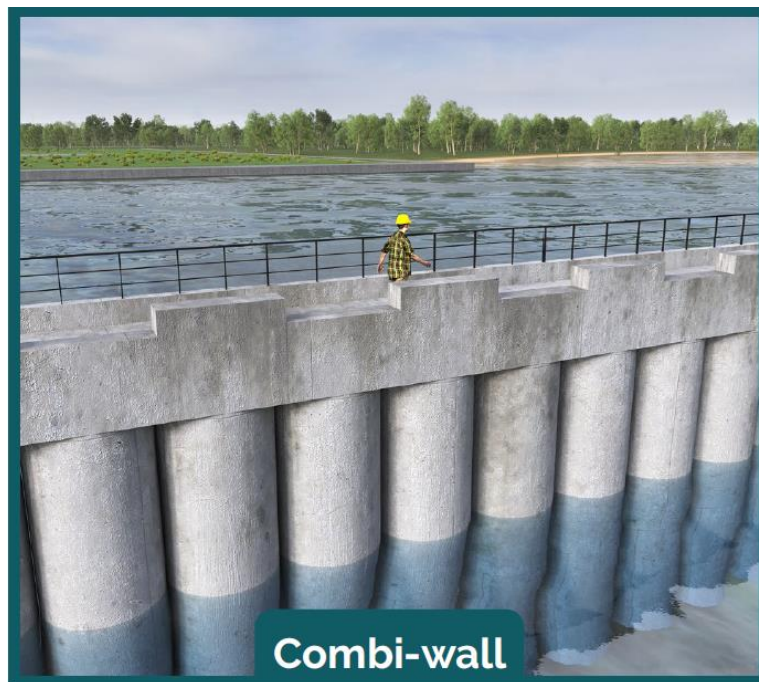
Figure 6-5: Combi-wall (Conceptual Rendition)
