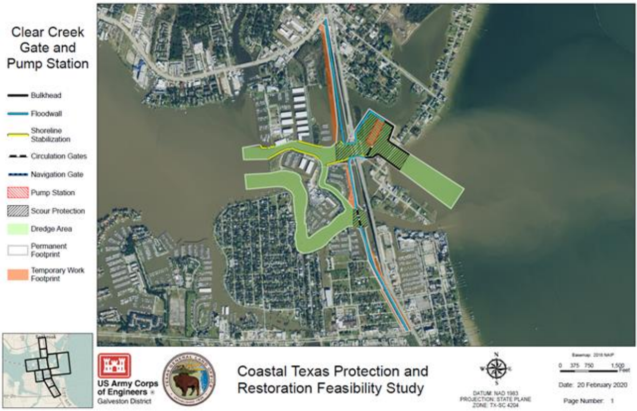
Figure 4-16: Clear Lake Gate Closure System
