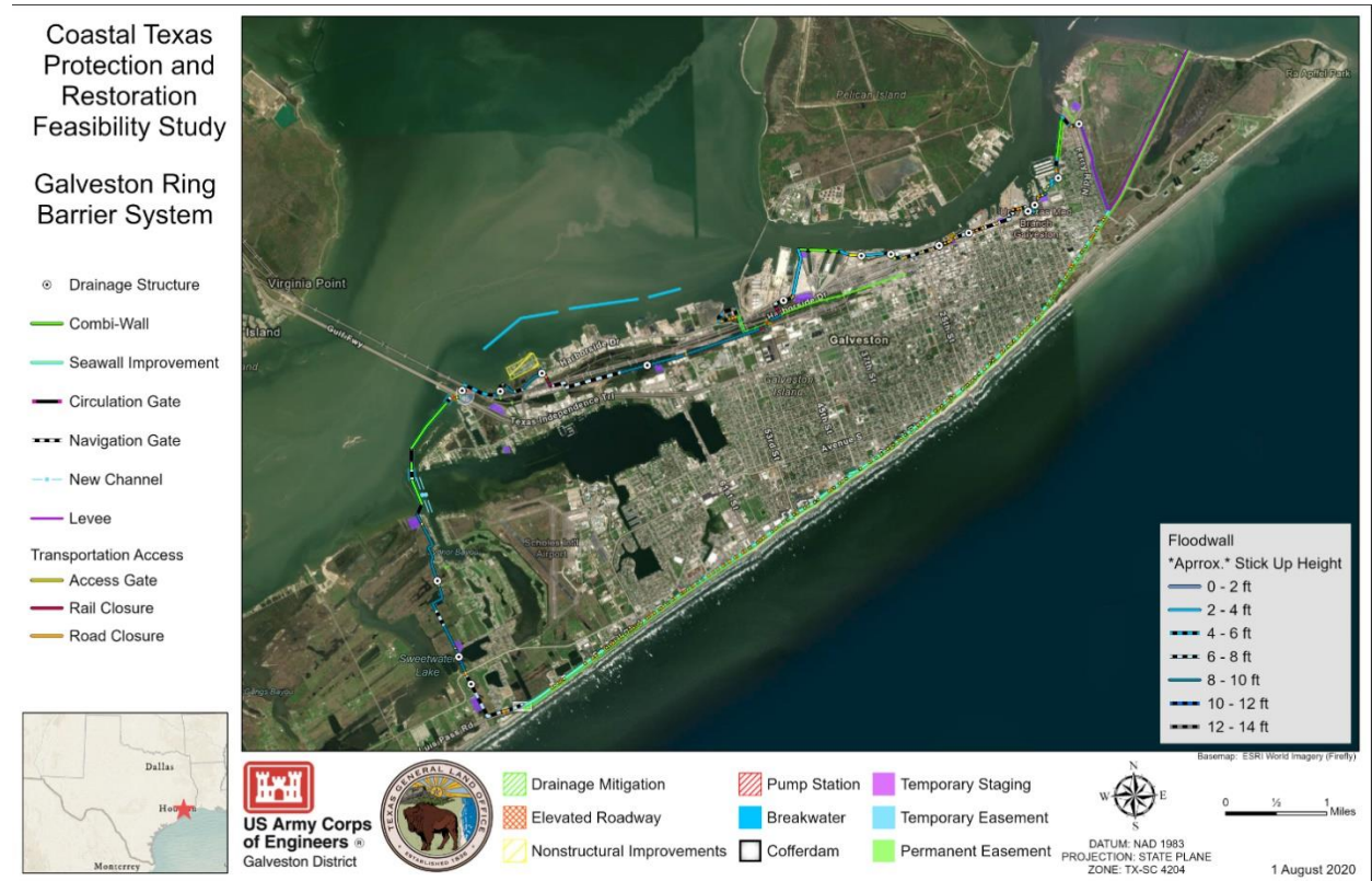
Figure 4-12: Galveston Ring Barrier System
